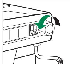
Switch on steam switch and wait for 10 min.
