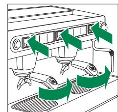
Lock the filter holder into the group head and switch on main switch
