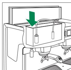
Connect the new softener to the tube and put it vertically in the tank
