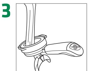
Rinse filter holder with hot water to dissolve any coffee bean oil residue
