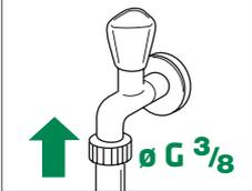
Connect fresh water tube (never crimp tube)
